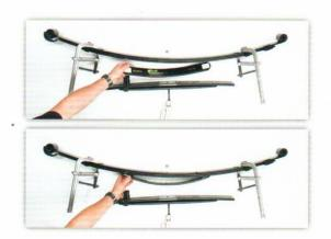
4. Gently tap the new centre bolt through the springs being careful not to damage the thread. Install the nut and tighten until moderate tension is felt.
