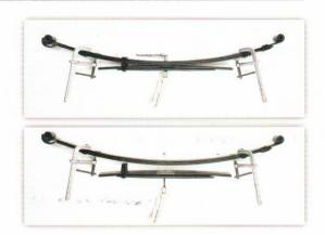
3. Carefully move the second stage away from the primary stage enough to add the Add-A-Leaf between the two stages and position the Add-A-Leaf as shown using the new centre bolt to align through the holes.
