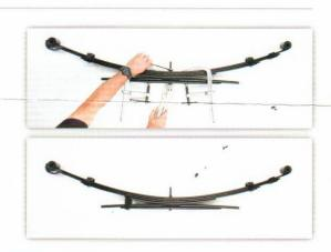
7. Wearing appropriate personal safety protection, use an angle grinder to trim the centre bolt leaving approximately 4 threads protruding through the nut and touch up the cut area with black paint to prevent rusting.
